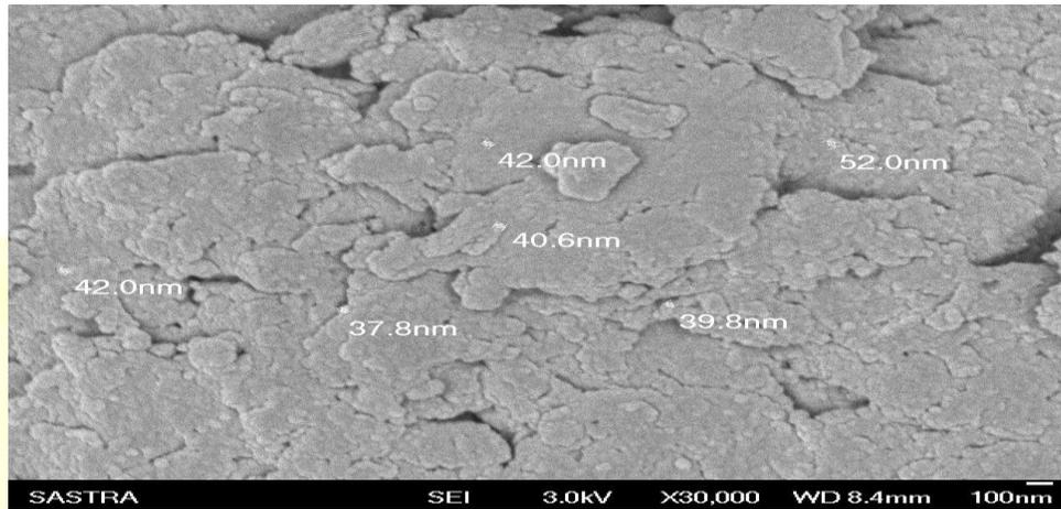
**Figure – 6 FESEM analyses of copper nanoparticles**
