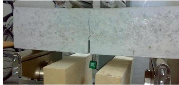
Fig 8.3 FLEXURAL STRENGTH TEST
