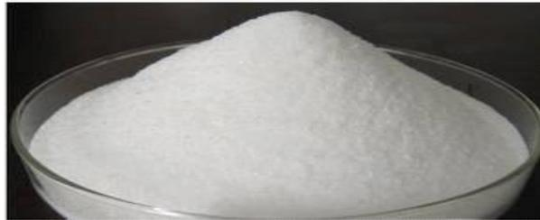
**Fig.5.6 Super Absorbent Polymer**
