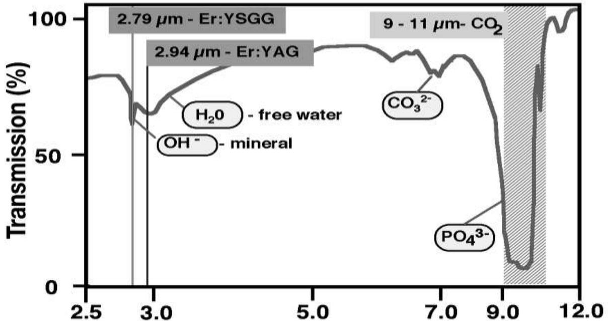
**Figure-5. Infrared transmission spectrum of dental enamel showing the position of the primary absorbers, namely phosphate ( $\text{PO}_4^{3-}$ ), carbonate ( $\text{CO}_3^{2-}$ ), hydroxyl ( $\text{OH}^-$ ) and water ( $\text{H}_2\text{O}$ ), together with the overlapping positions of the Er:YSGG, Er:YAG and carbon dioxide (9.3, 9.6, 10.3 and 10.6  $\mu\text{m}$ ) lasers [37].**
