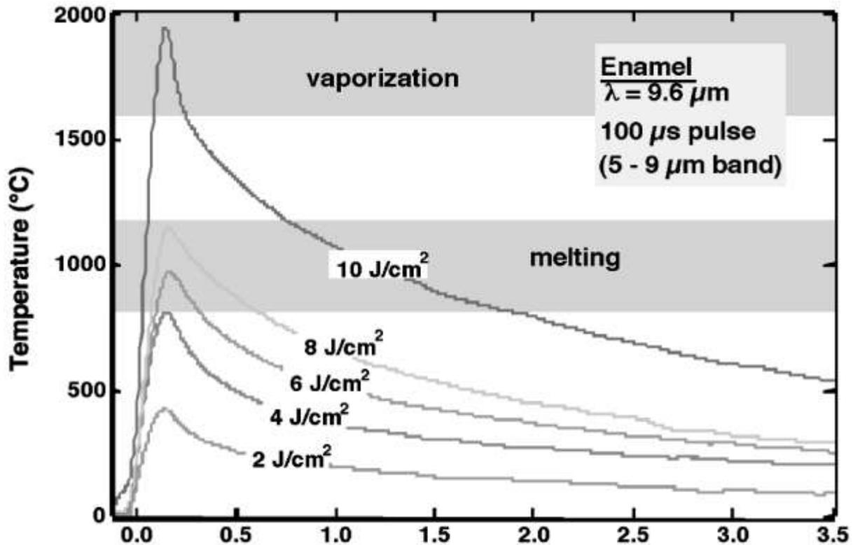
Figure- 4. Plot of temperature at the surface of dental enamel versus time following irradiation by a carbon dioxide laser at 9.6 μm , over a range of fluences and with pulse duration 100 μs (11).
