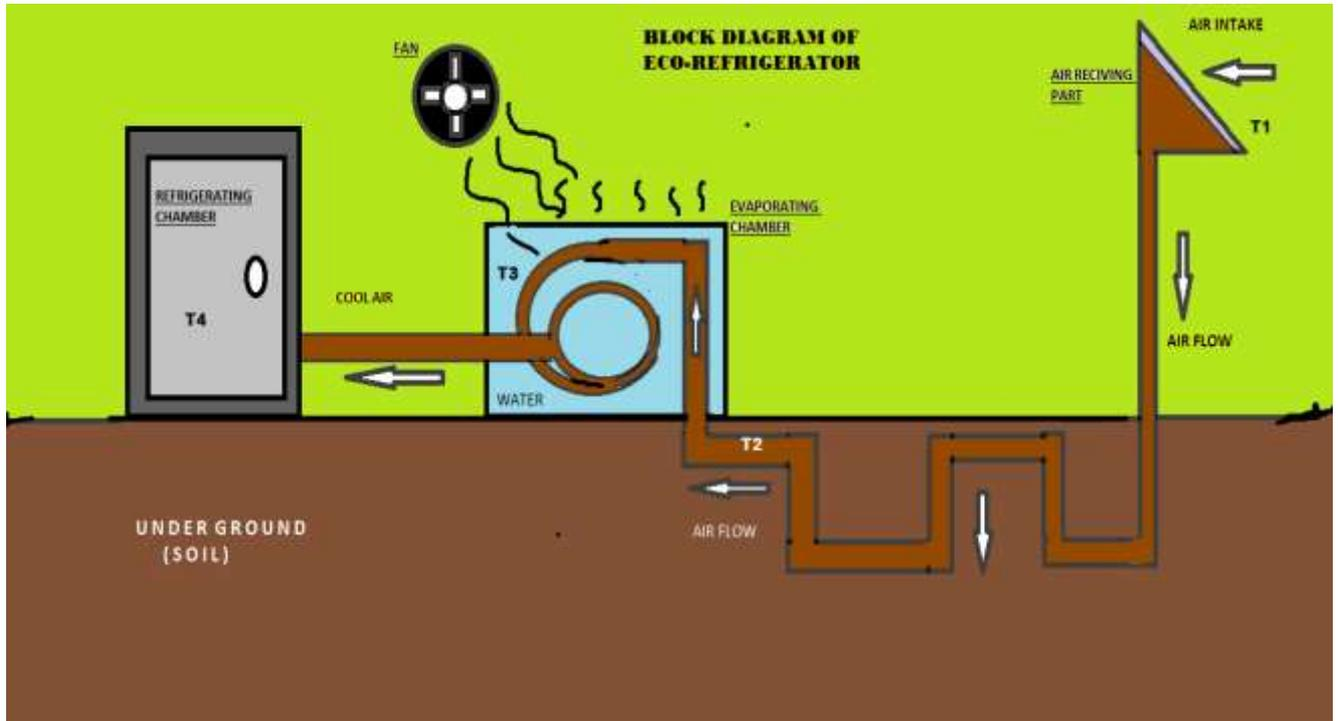
Fig1:- Block diagram of Eco-Refrigerator
