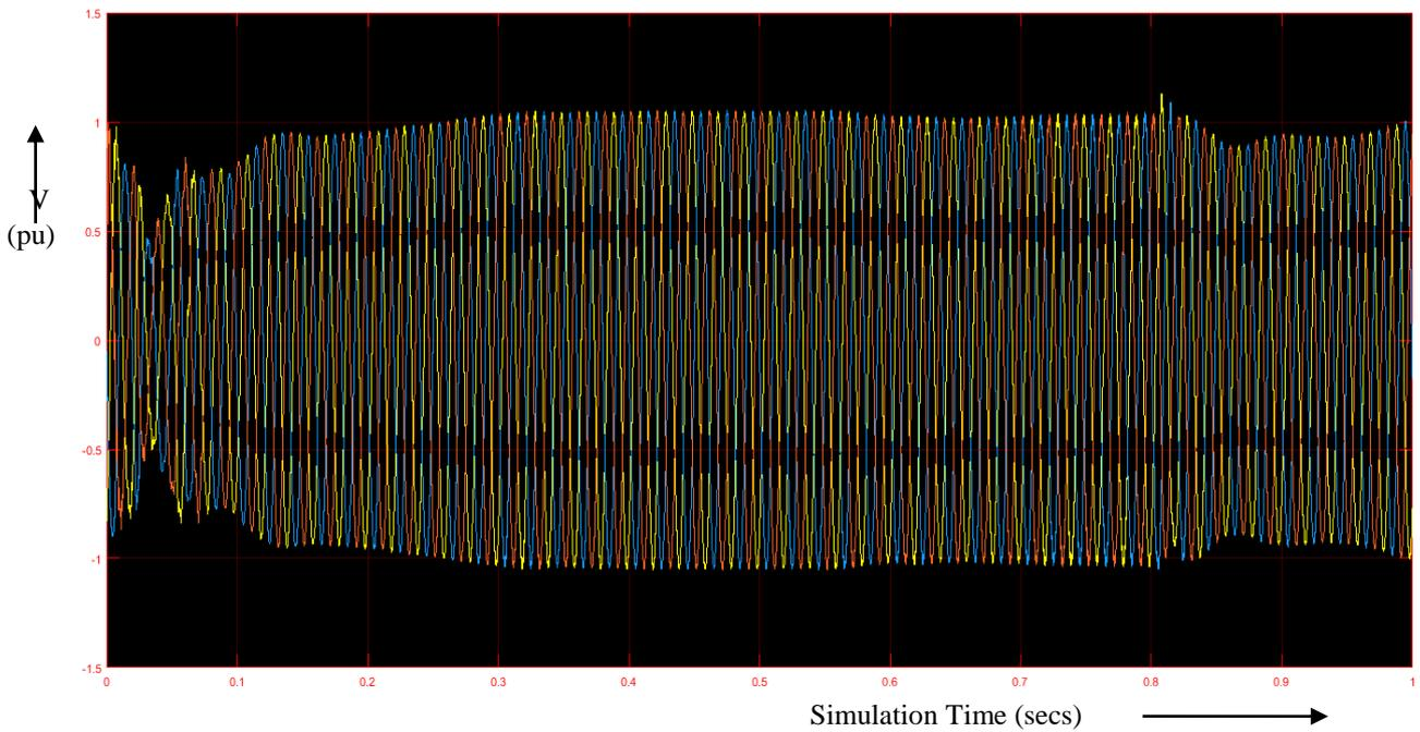
**Fig.7.2: Voltage response for Yola bus at P<sub>max</sub> with a three phase fault and with UPFC and CCC-HVDC connected.**
