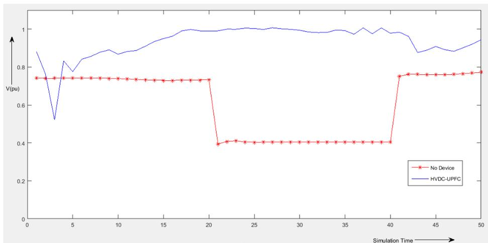
**Fig. 7.3: A graph of peak phase voltage profiles (with and without devices) against simulation time at Yola Bus with three phase fault contingency imposed on the network**
