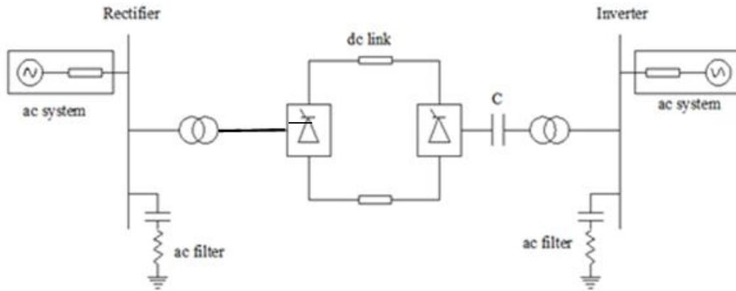
**Fig 4.1: Schematic diagram of a CCC-HVDC. [7]**
