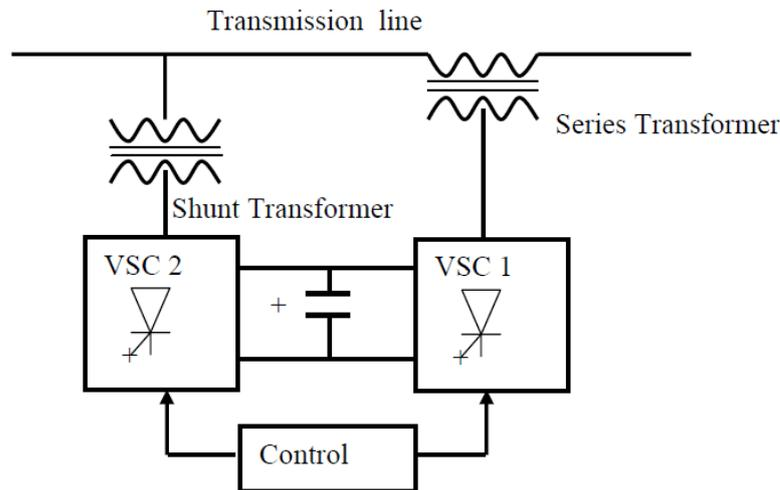
**Fig 3.1: Schematic diagram of a Universal power flow controller (UPFC) [5]**
