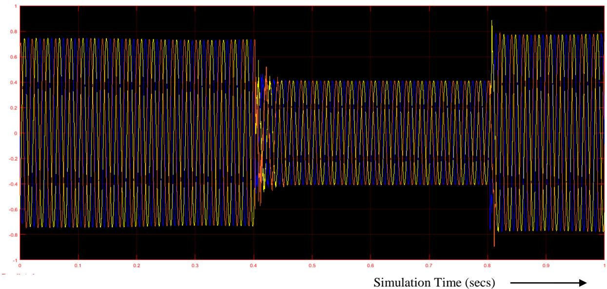
**Fig.7.1: Voltage response for Yola bus at  $P_{max}$  with a three phase fault with no device connected**
