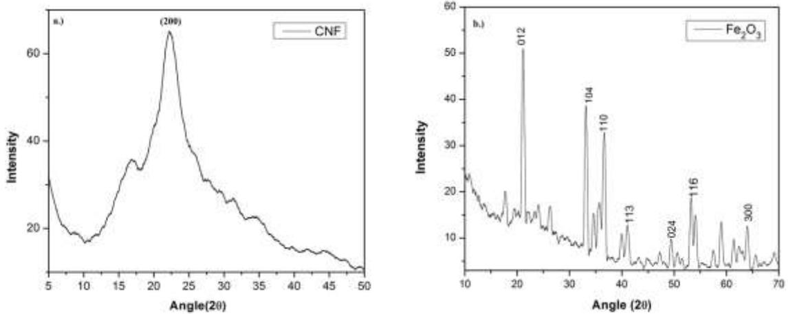
**Figure 1a) X-ray diffraction spectra of cellulose nanofibers, 1b) X-ray diffraction spectra of iron oxide nanocubes.**
