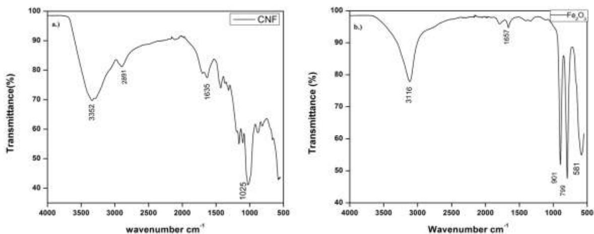
**Figure 3a) FTIR spectra of cellulose nanofibers, 3b) FTIR spectra of iron oxide nanocubes.**
