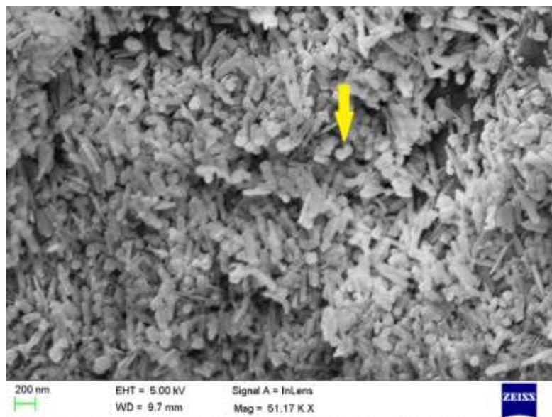
**Figure 2: SEM image of cellulose nanofibers and iron oxide nanocubes**
