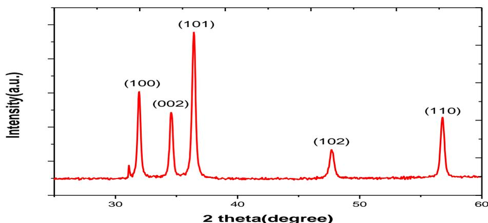
Fig.1: XRD pattern of single layer ZnO film annealed at 400°C for 1 h in air.
