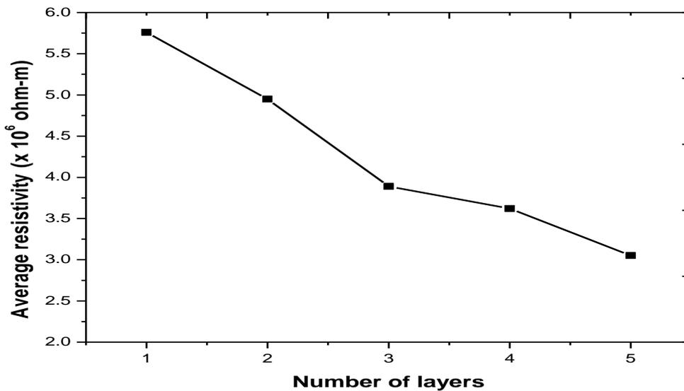
Fig. 4: Variation of average resistivity of ZnO film with number of layers.
