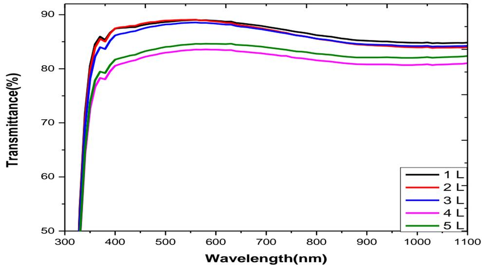
Fig. 2: Optical transmittance spectra of multi-layer ZnO thin films annealed at 100°C in air.
