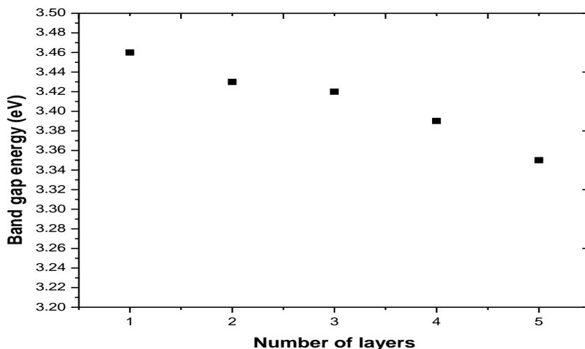
Fig. 3: Variation of optical band gap energy of ZnO film with number of layers.
