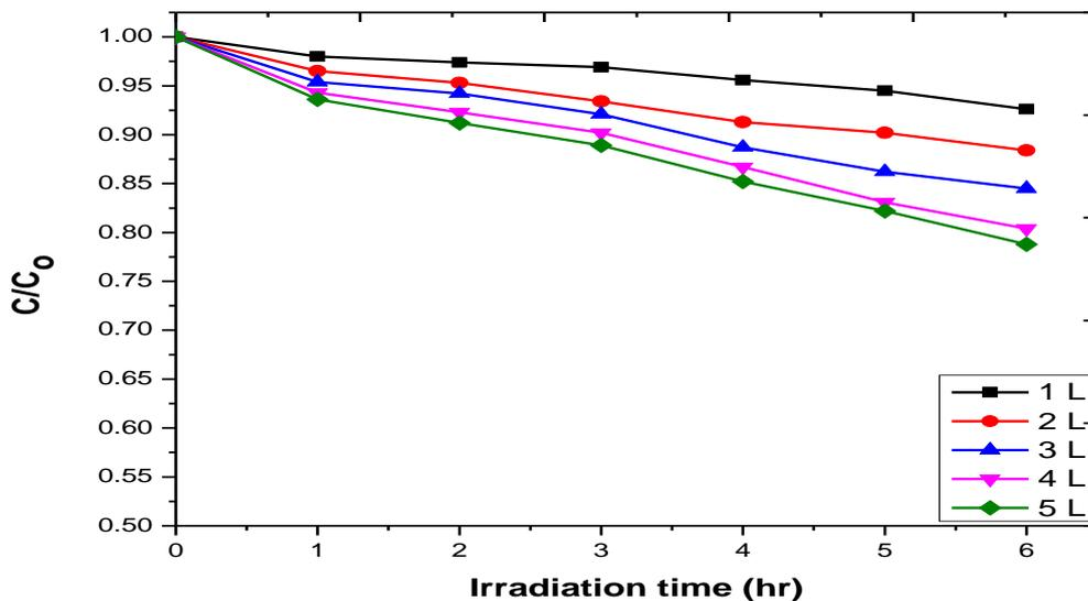
Fig.5: Photo-catalytic degradation of rhodamin B dye using multi-layer ZnO films.
