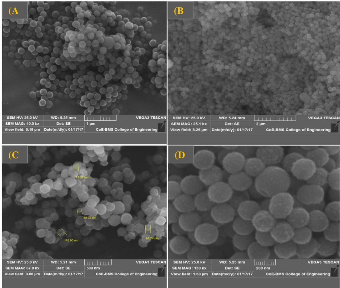
Figure 2:(a) SEM images of (A) Si Colloid, (B) Thiol capped Si Colloid and (C) Co NPs, (D) Silica supported Co NPs and (E) EDX pattern of silica supported Co NPs.
