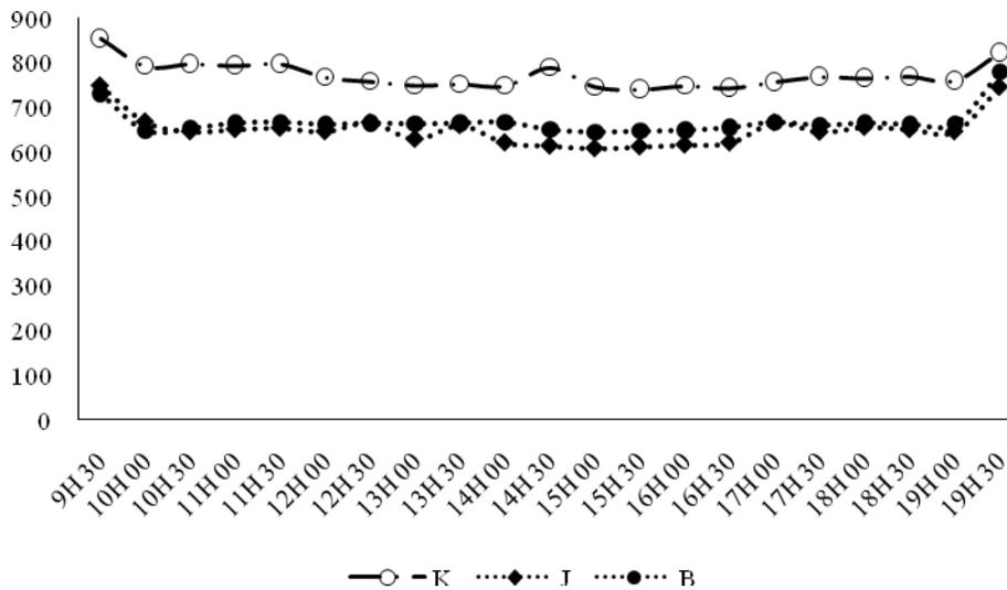
Figure 7. Load profiles in a cab whose subscribers do not use prepayment meters. The curves of the load profiles are very dynamic in the mixed cabins. Significant variations are observed during the hours observed. The low consumption represents 201A while the high represents 371A.
