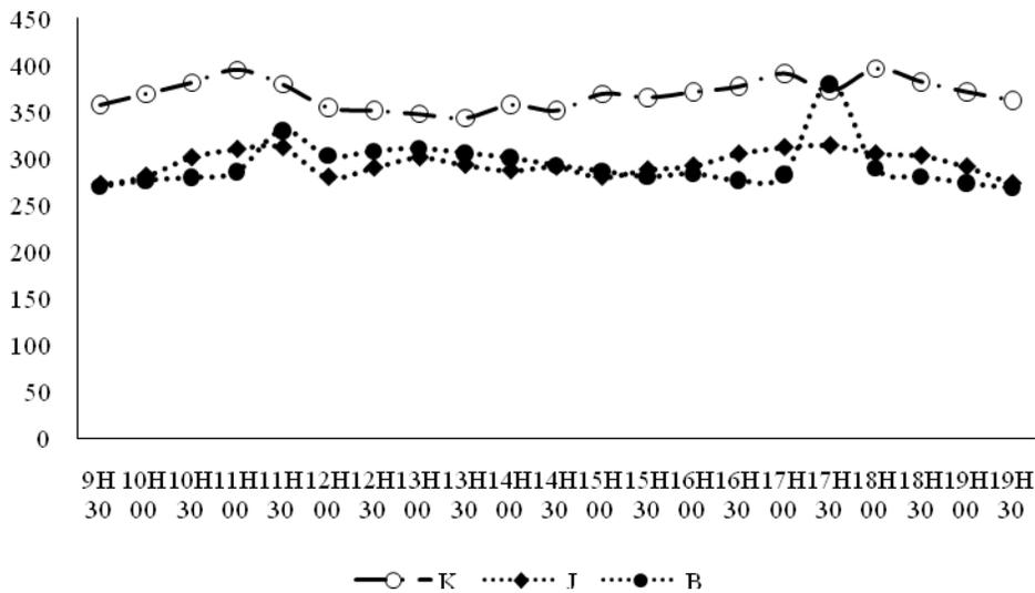
Figure 5. Load profiles in a cab whose subscribers do not use prepaid meters. In the cabins with prepayment meters, the highest consumption is 230 A while the lowest is 165 A. The consumption values in the meter cabs seem to be much lower compared to the values observed in the mixed cabins a share and post-payroll.
