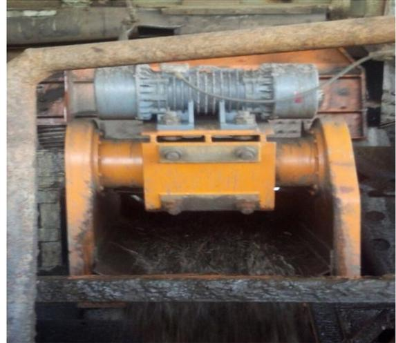
Figure 1: CHEMAF Vibrating Feeder
