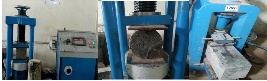
Figure 2: Testing methods for the strength of concrete
