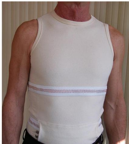
*Figure 7.* Textile sensors for Kinematic Analysis<sup>[52]</sup>
