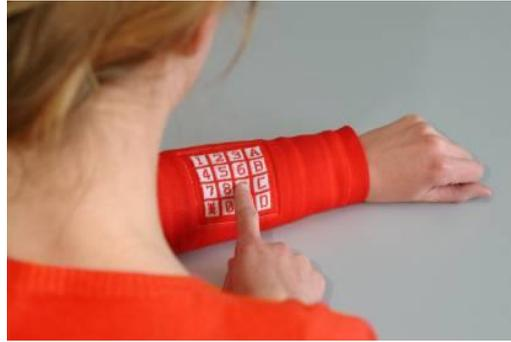
**Figure 8.** Realizing pressure sensors using textile process e.g.: Keyboard<sup>[45]</sup>
