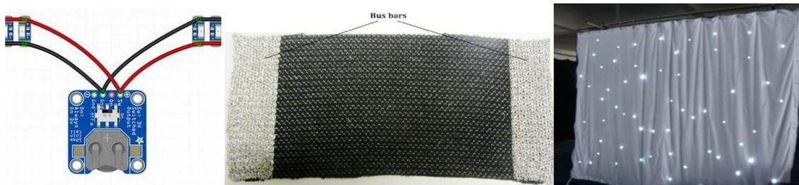
**Figure 3.** (Left) Adafruit coin cell battery holder. The first generation saw devices attached to textiles. (Middle) Knitted electrodes. The second generation of electronic textiles describes functional fabrics in which conductive elements are integrated into textiles. (Right) Example of functional thread (in this case LED Thread). The third generation of electronic textiles describes electronics embedded in textiles at thread level <sup>[7]</sup>.
