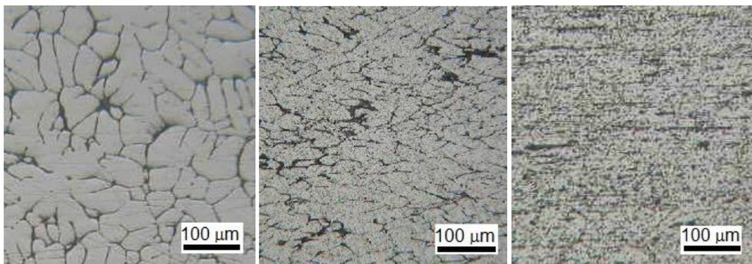
Fig.2. Optical micrographs of composites of AlZrCe (Zr = 0.15%, Ce = 0.2%) alloy reinforced by nanoparticles of Al<sub>2</sub>O<sub>3</sub> (1.2% volume fraction) (a) as-received (as-cast), (b) after hot rolling (450 °C, r = 51%), and (c) followed cold rolling (r = 70%) in rolling direction.
