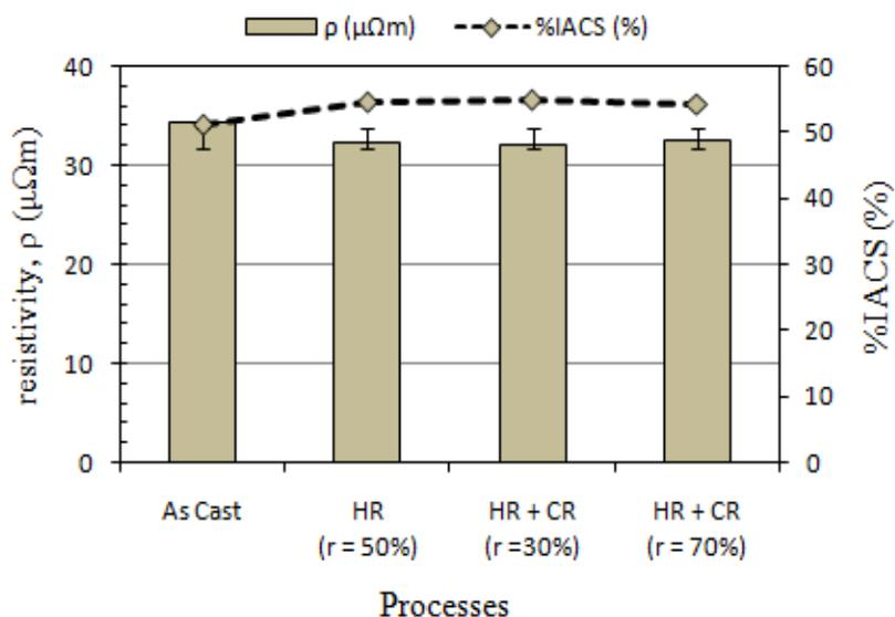
Figure 6. Electrical conductivity of the MMC samples of AlZrCe alloys reinforced by alumina particles before and after hot rolling (50% reduction) and cold rolling (70% reduction).
