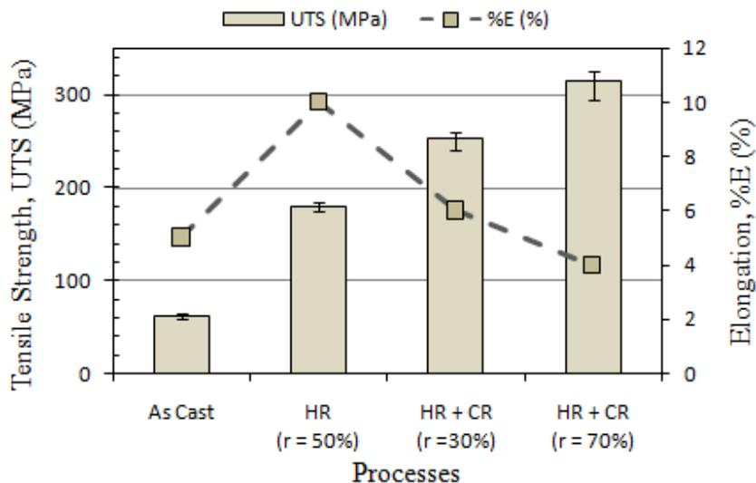
Figure 5. Tensile strength and elongation of the MMC samples of AlZrCe alloys reinforced by alumina particles before and after hot rolling (50% reduction) and cold rolling (70% reduction).
