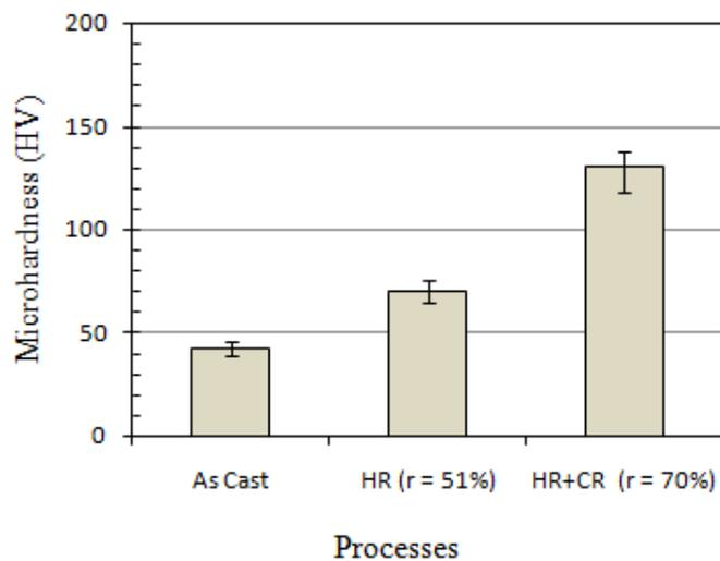
Figure 4. Hardness of MMC samples of the MMC samples of AlZrCe alloys reinforced by alumina particles before and after hot rolling (50% reduction) and cold rolling (70% reduction).
