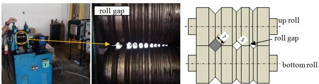
Figure 1. Rolling mill for hot rolling and cold rolling with several size (square) profil gap
