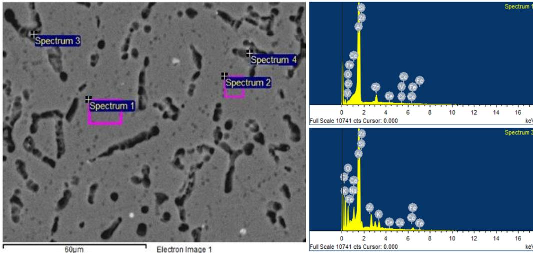
Fig.3. SEM micrograph of composites of AlZrCe alloy reinforced Al<sub>2</sub>O<sub>3</sub> nanoparticle in cross section after hot rolling (a) and its EDs analysis.
