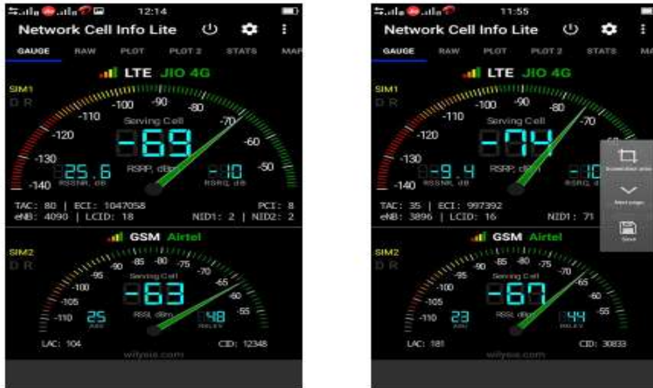
Figure 1. Mobile app. 'Network Cell Info Lite' used to measure signal strength at 100 m from the tower in dBm. Value close to zero indicates stronger signal
