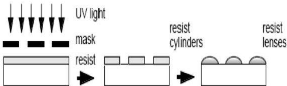
Figure 1: Demonstrates the formation of Micro lens Array by the combination of photolithography and thermal reflow process.
