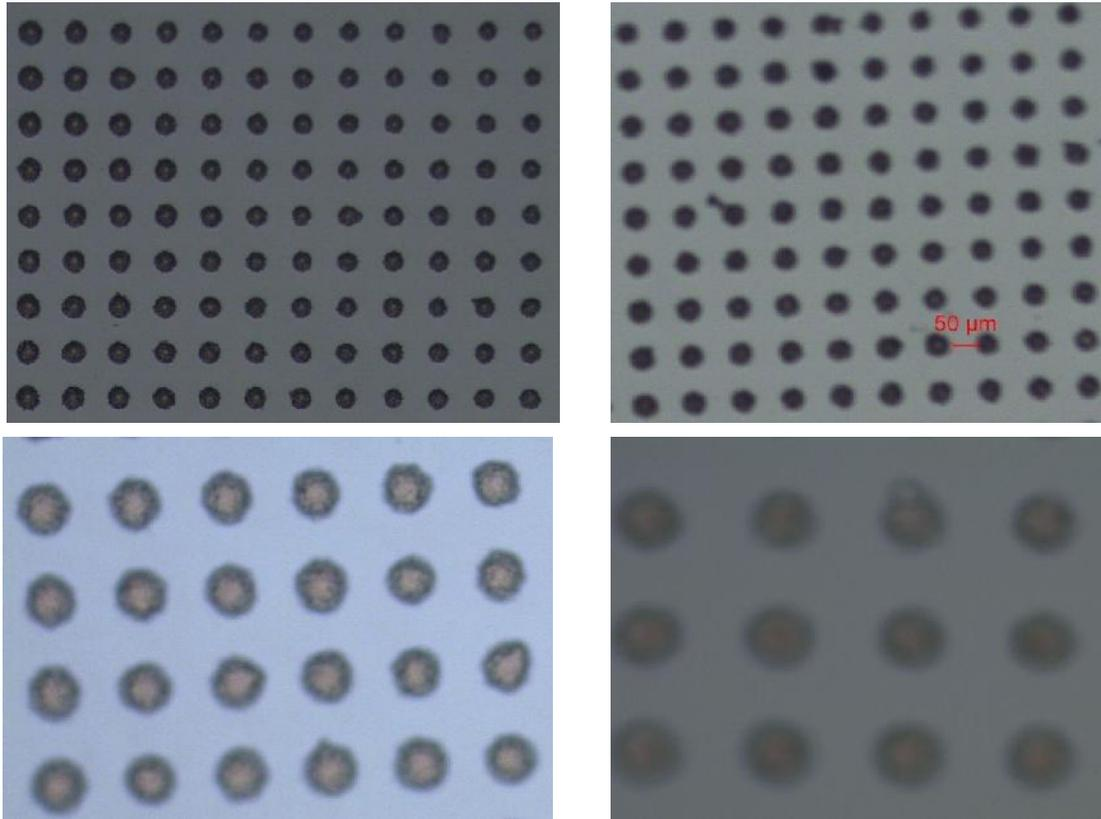
**Figure 4: Optical microscope images of dot arrays on photoresist with 50  $\mu\text{m}$  diameter and 50  $\mu\text{m}$  spacing between the circle at different magnification. These are the images before photoresist reflow.**
