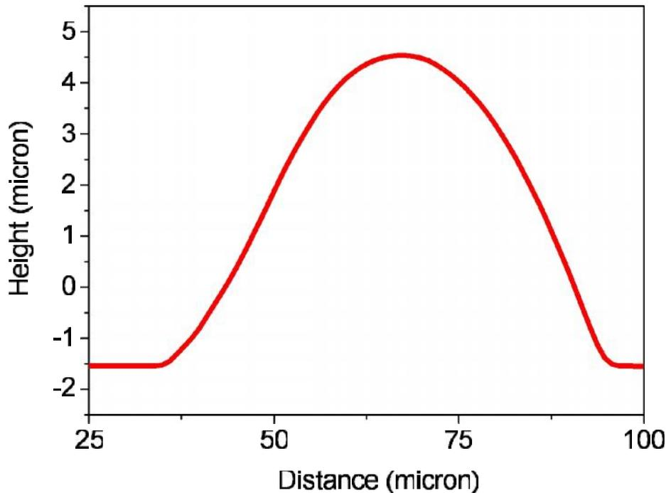
**Figure 7: Sag height after thermal reflow**
