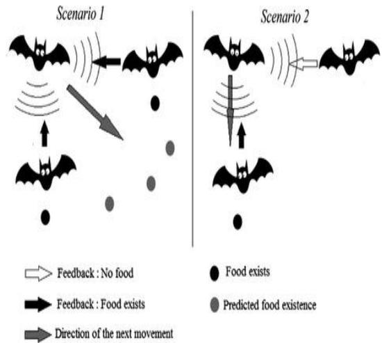
Fig. 6. Bat Algorithm and Directional Bat Algorithm [13]
