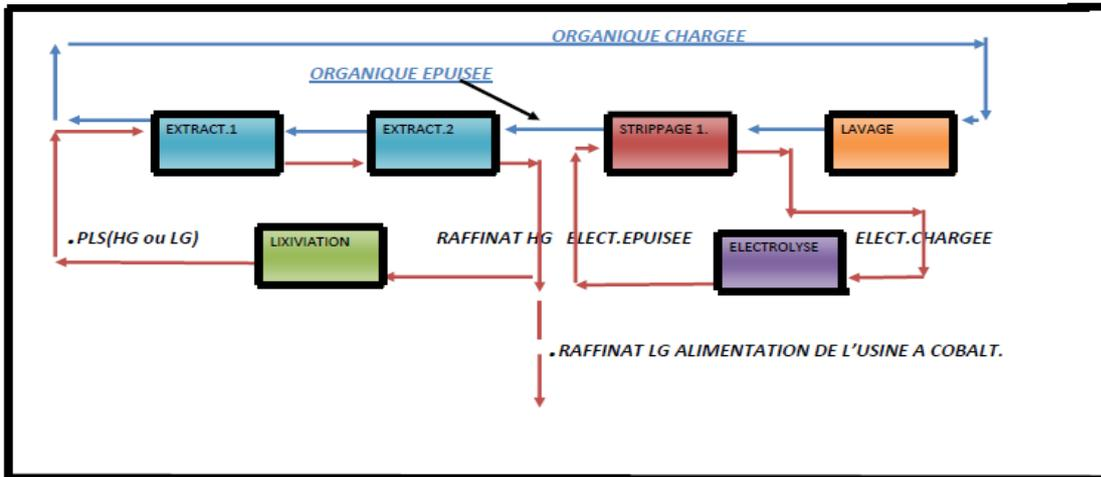
**Figure 10: Schematic of Solvent Extraction**
