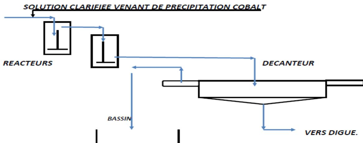
Figure 14 : Magnesium precipitation circuit
