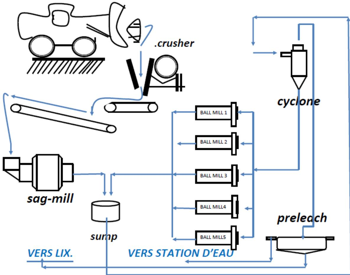
**Figure 6 : Schematic of the fragmentation circuit**
