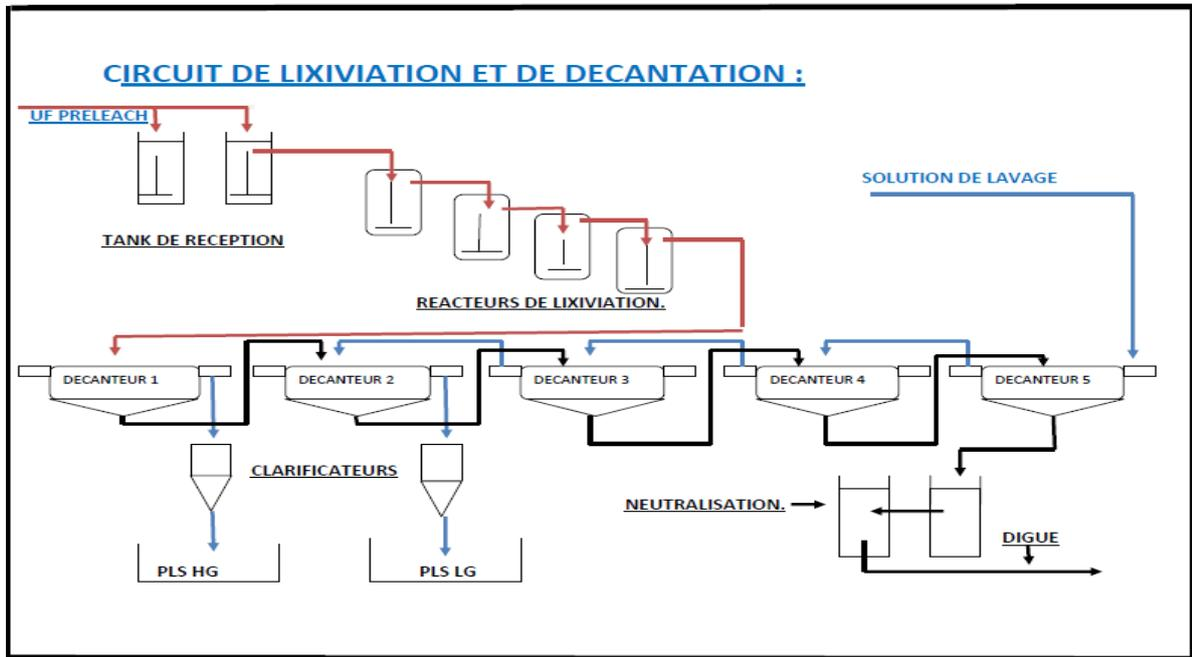
Figure 7: Leaching and settling circuit
