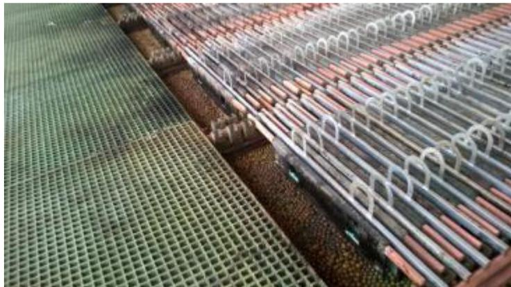
**Figure 12: Pellets against gassing at electrolysis.**
