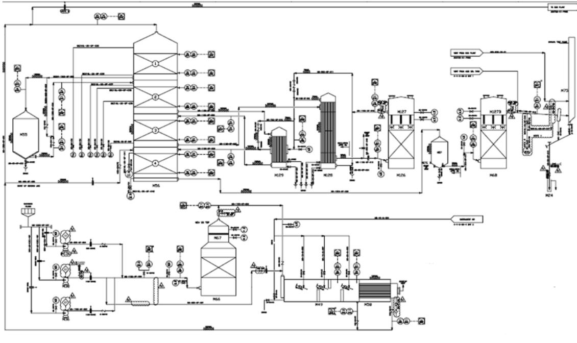
**Figure 16 : Flow-sheet of the sulfuric acid plant**
