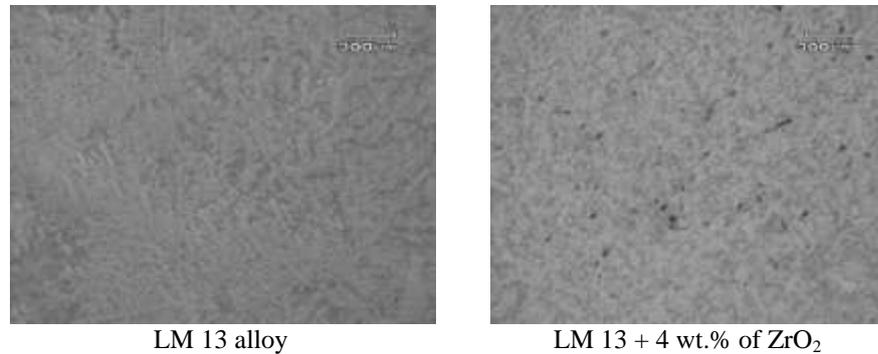
Figure 3: Optical micrographs of as-cast aluminium alloy and aluminum (LM13)-nano ZrO<sub>2</sub> MMCs
