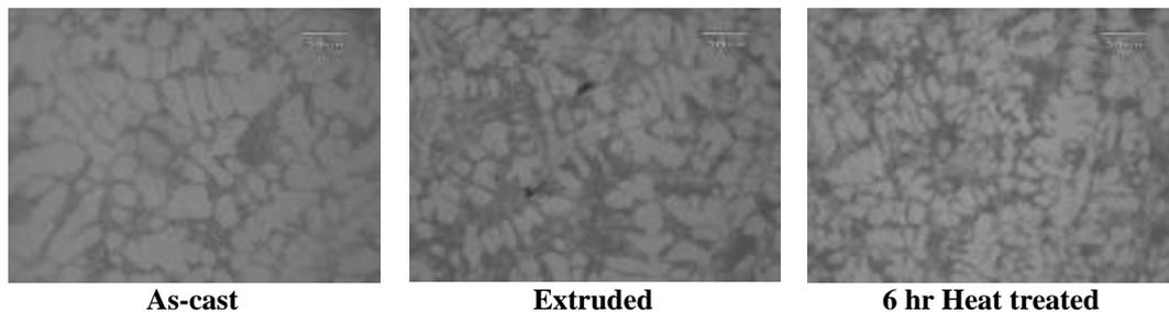
Figure 4: Optical micrographs of as-cast, extruded and heat treated LM13-2 wt.% nano ZrO<sub>2</sub> MMC
