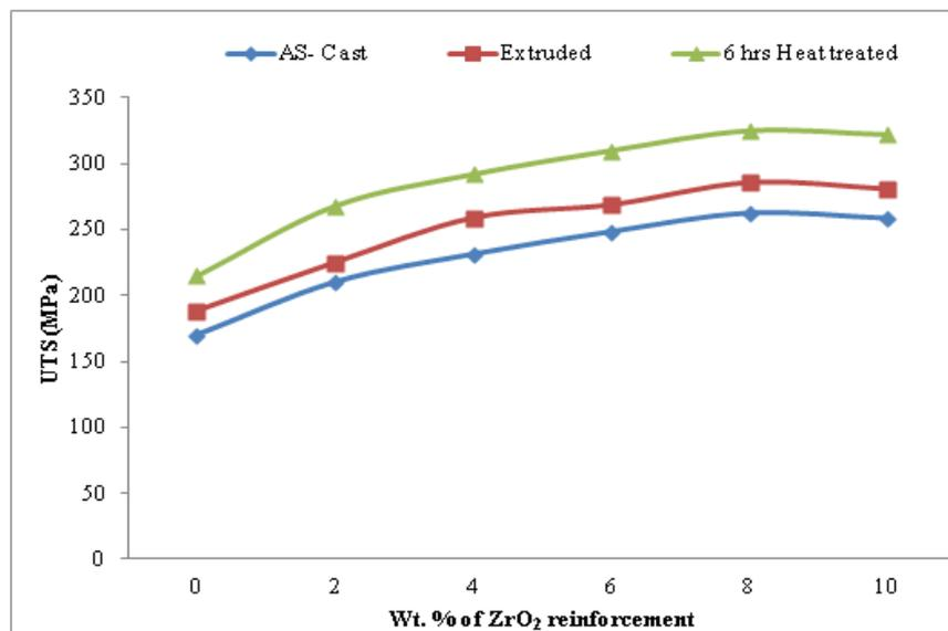
Figure 7: Influence of extrusion and heat treatment on UTS of the LM13-nano ZrO<sub>2</sub> MMCs
