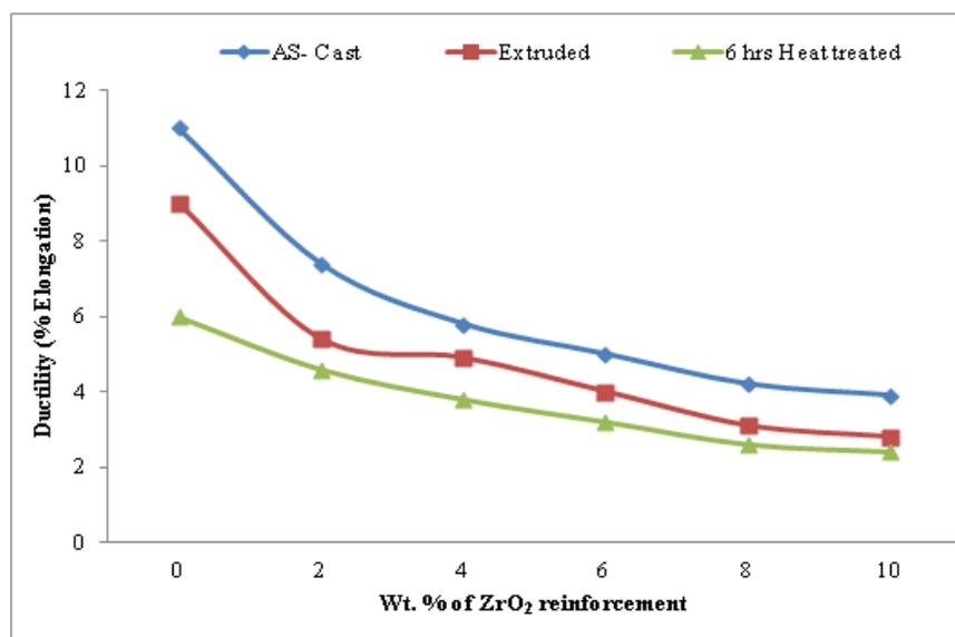
Figure 9: Influence of extrusion and heat treatment on ductility of the LM13-nano ZrO<sub>2</sub> MMCs
