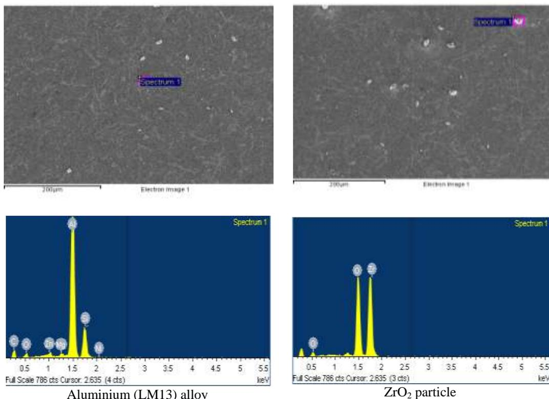
Figure 2: SEM photographs and EDAX pattern of Aluminium (LM13) alloy and ZrO<sub>2</sub> particle in MMC
