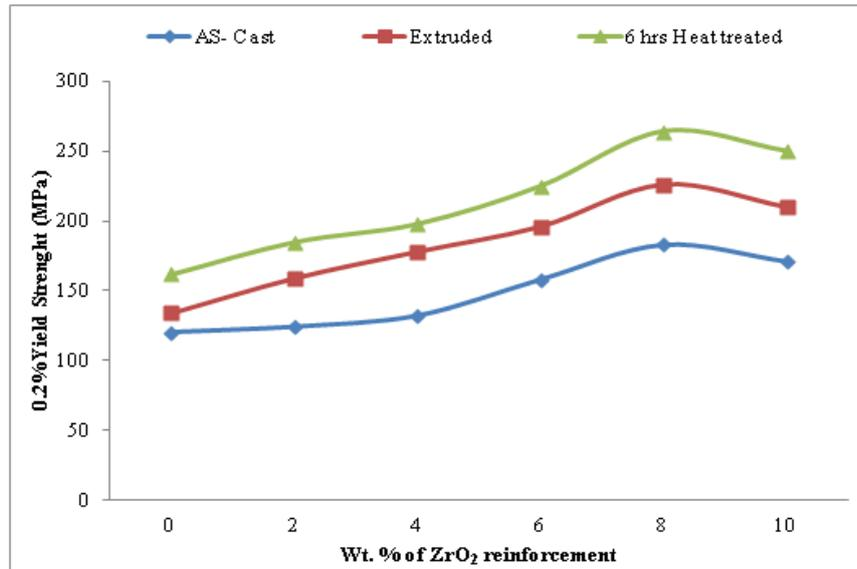
Figure 8: Influence of extrusion and heat treatment on yield strength of the LM13-nano ZrO<sub>2</sub> MMCs
