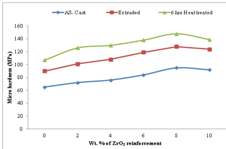
Figure 6: Influence of extrusion and heat treatment on micro hardness of the LM13-nano ZrO<sub>2</sub> MMCs
