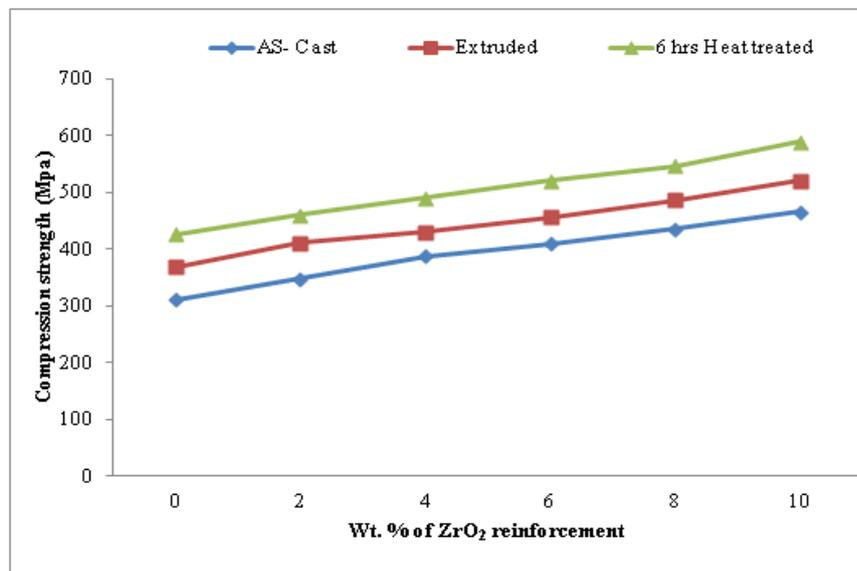
Figure 10: Influence of extrusion and heat treatment on compression strength of the LM13-nano ZrO<sub>2</sub> MMCs
