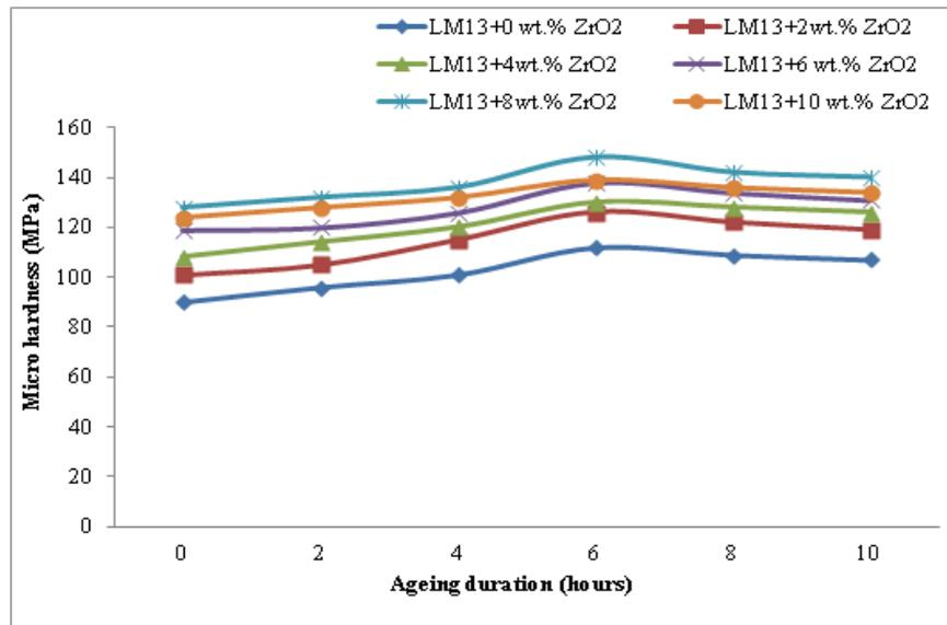
Figure 5: Influence of heat treatment on micro hardness of the extruded LM13-nano ZrO<sub>2</sub> MMCs
