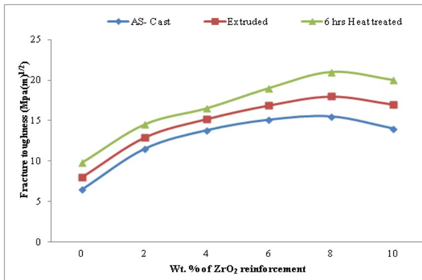
Figure 11: Influence of extrusion and heat treatment on fracture toughness of LM13-nano ZrO<sub>2</sub> MMCs
