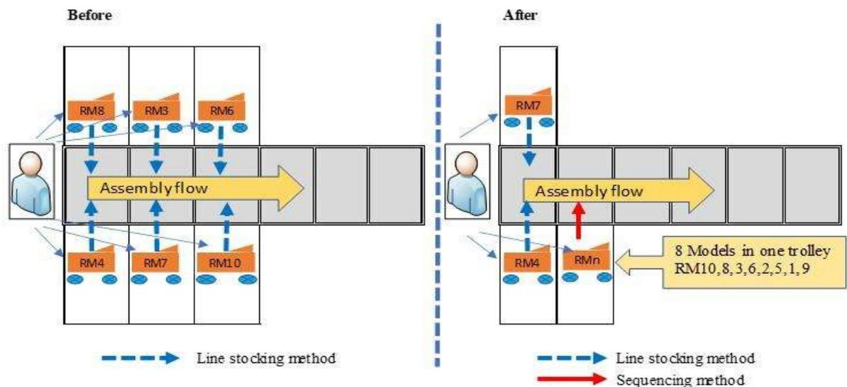
After changing the method of feeding at line border the movement of operator (Start- Go- Pick- Return) cycle is reduced from 2304 secs to 1600 secs per shift, it is about 704 secs reduction (31%) compared to the previous feeding method (Line stocking).
