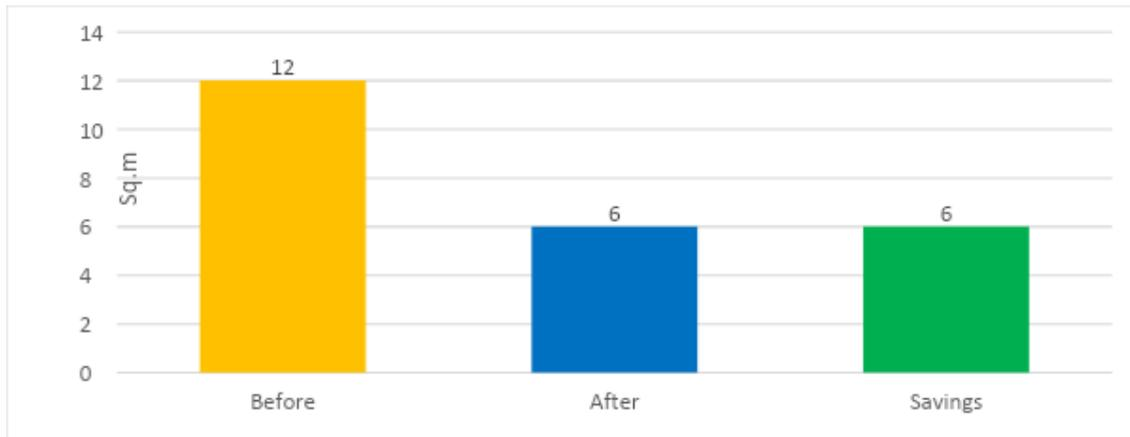
Previously the assembly line border occupied with 6 trolleys which was occupied 12 Sq.m of space and after implementation of new hybrid feeding method, it has been reduced to 6 Sq.m
