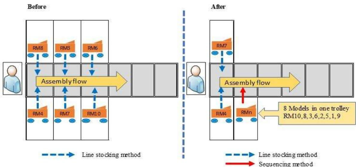
Previous condition was the individual model parts per trolley in full kept near by the line borders, proposed condition only two trolleys of majorly runner parts kept in line border in full and other models new production orders were kept in a single trolley on sequence flow method
