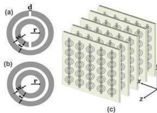
Figure 4 . Schematics of (a) a single split ring resonator(SRR) (b) a ring resonator with splits closed (CSRR) (c) PeriodicCMM composed of SRRs on one side, wires on the other side of dielectric board.
