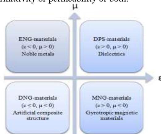
Figure 1: The general classification of physical materials depending on values of permittivity( $\epsilon$ ) and permeability( $\mu$ )
