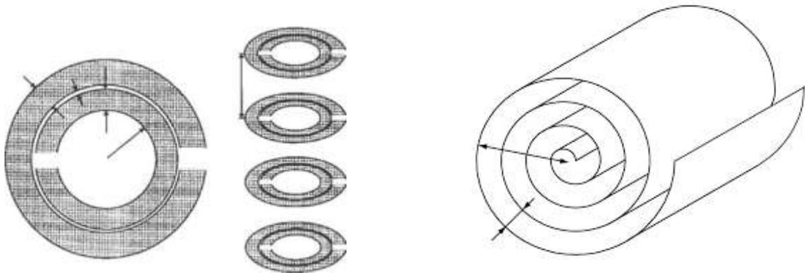
Figure 2.(a) SRRs in the 1990s. (From Pendry, J.B., Holden, A.J., Robins, D.J., and Stewart, W.J., *IEEE Trans. Microw. Theory*, 47, 2075, 1999) (b) Swiss rolls. (From Hardy, W.N. and Whitehead, L.A., *Rev. Sci. Instrum.*, 52, 213, 1981 ; Wiltshire, M.C., Pendry, J.B., Young, I.R., et al., *Science*, 291, 849, 2001)
