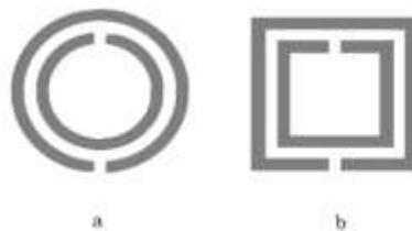
Figure 3. The first MNG-material unit cells: a) round, b) square
