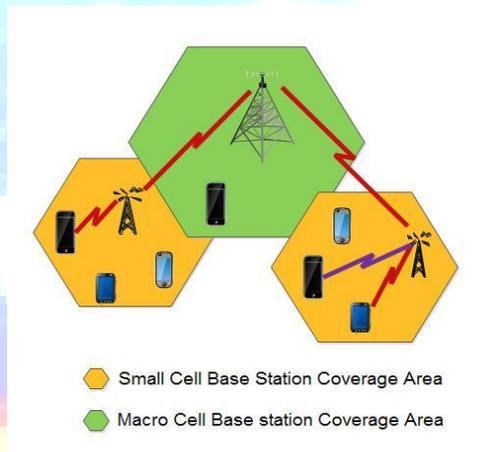
Fig.4 Interference due to Multiple Transmissions.
