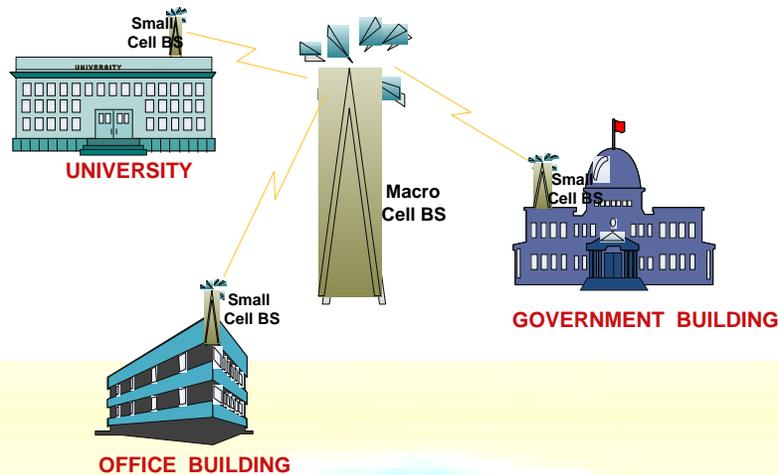
Fig.1 Heterogeneous Deployment of small cell Networks
