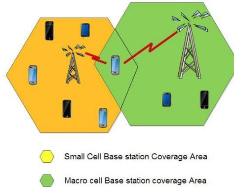
Fig.3 Interference occurs a single user is served by both small cell and macro cell Base stations.
