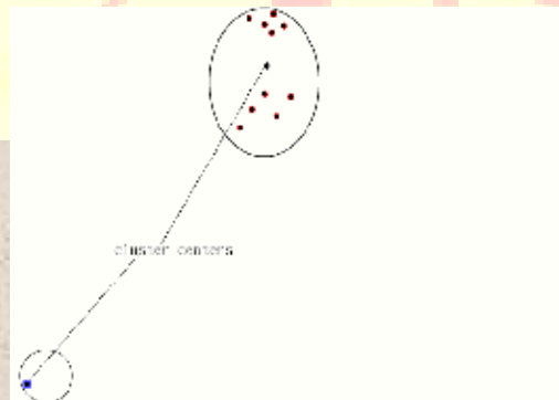
(d) Clustering result from the FCM algorithm with an outlier on the left.
