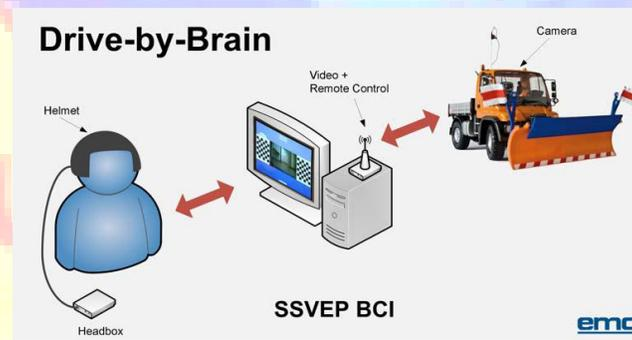
Fig.1: The control of machines by means of steady-state visually evoked potentials is done via the helmet, which records the brain signals and transmits them to the computer. It evaluates the signals and controls the vehicle via remote control.
