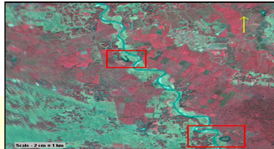
Fig. 6 Ox-bow lakes giving rise to very dark grayish green tone on the LISS-III 1C/1D image- a part of Bhogdoi River.
